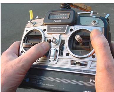
Leaving the throttle stick in the minimum position, raise the throttle trim to the max position or switch "Engine Cut" switch to off, and again press the + button.
