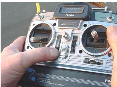
Move the throttle trim (or switch the "engine cut" switch to on) and throttle stick back to zero and again press the + button.
