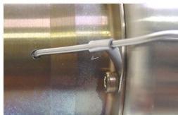
The temperature sensor is pre-shaped and retained in the exhaust cone by the small bracket which is secured to one of the exhaust cone screws. It should protrude approx 4mm through the small hole at 3 O-clock in the exhaust cone (viewed from the turbine end).
