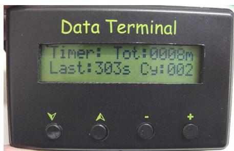
The “INFO” screen of the ECU display contains a timer which shows the total running time of the engine in minutes, the number of starts (cycles - CY) and the time in seconds of the last run.
